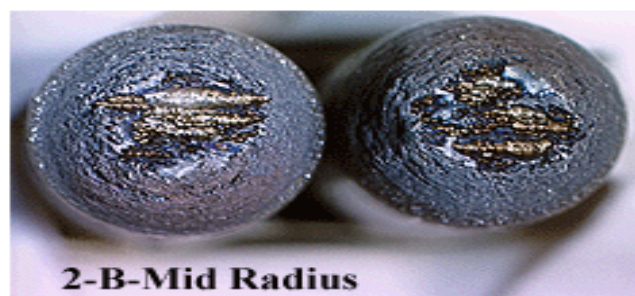
Figure 5.1: Fractographs, Comparison of Run 1, 2200 F
